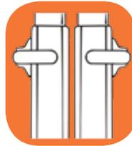
**WARNING: DO NOT USE LADDER WITH DAMAGED OR REMOVED SAFETY STRAPS. FAILURE TO HEED WARNING MAY RESULT IN INJURY.**
