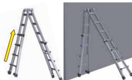
From the tall A-frame position, reduce the height on one side of the ladder by one rung. Make sure the ladder is on a flat level surface and the short side is against a secure wall.
