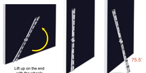
Open and lock your ladder into the extension position, and lay it face up on the ground with the feet near the wall. If your ladder has wheels, they should be on the end farthest from the wall. Unlock the Rapid Locks on the top outer section and extend it to the desired height, locking both Rapid Locks when finished. If you need more height, repeat this for the bottom section as well.
