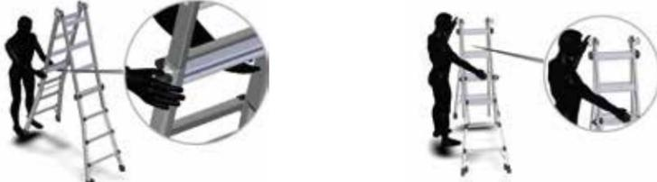
To bring the ladder down from the A-frame position, place one hand under the inner and outer rungs to secure the ladder from moving. With your other hand, unlock one Rapid Lock, then switch hands and unlock the other one. Next, place your hand on the Palm Button to hold the inner section in place before you remove your hand from keeping the inner and outer section secure.
