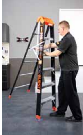
COMPLETELY OPEN THE LADDER
