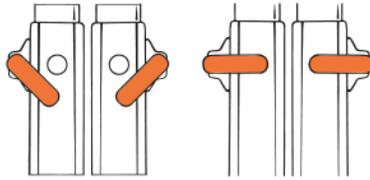
The Lock Tabs adjust the height of ladder. Pull out the Lock Tabs to unlock, replace the Lock Tabs in the desired rung tube. Unlock only one Lock Tab at a time while supporting the inner ladder assembly with one hand. Do not unlock the Lock Tab if any one is on the ladder.
