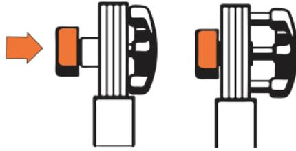
Push the Palm Buttons in to release the hinge locks.
